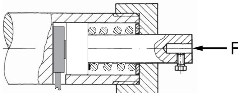
Figure 5: Mounting of 8438 using initial load
